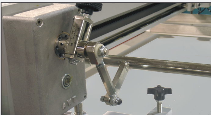
Exclusive upfront peel system gives operator quick and convenient control of peel rate setting.
